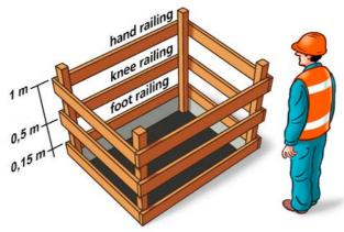
In some cases it may be necessary that the top handrail is higher and stronger then usual. For example, the handrail on a work platform encounters a sloping roof. If the railing is higher it may need another handrail added. In some instances, it may also be necessary that the railings are covered in netting to prevent small items and materials from falling.
