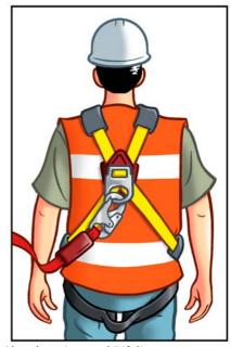
Harness and Fall Arrest Shock Absorbent Lanyard/Lifeline
